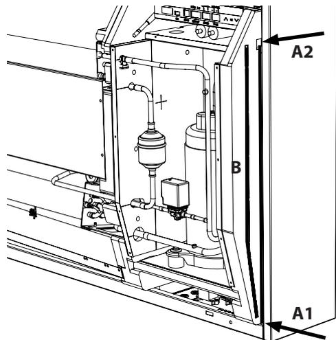
Two cable grooves for accessory make it easy to guide the cables from the control panel to the mains electricity connection and out of the unit.
