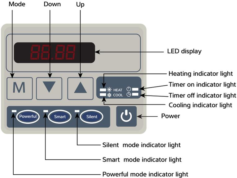
Note: When the heat pump is powered off, the display shows the time.
