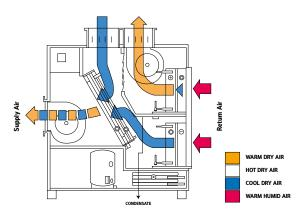
Delta models 4 and above provide an air conditioning facility to minimise the effects of solar gain from larger glazed areas or very high usage. Automatic damper and mode control.
