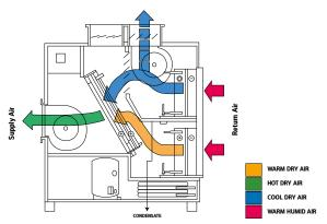
Air temperature set back control is incorporated as standard in all Delta units and controlled by a time clock. Pool hall air is dropped to a lower temperature for maximum economy. Air recirculation is maintained, dampers allow low fresh air flow.
