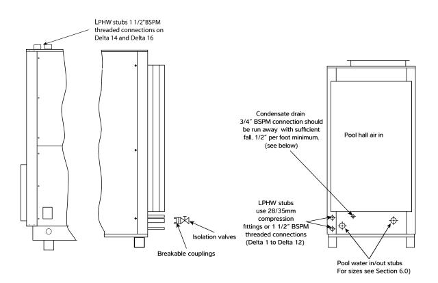
Fig 3.1 Condensate drain schematic
