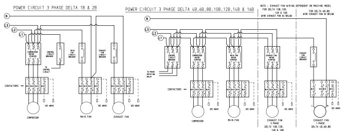
FOR DELTA 4B, 6B, 8B, EXHAUST FAN SETTING DENOTES RATING FOR SINGLE POLE MCB CIRCUIT BREAKER
