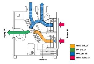
Delta operating on light dehumidification with full heat recovery and reduced fresh air stream – control system automatically selects correct operating mode and damper position. LPHW heat available when required.
