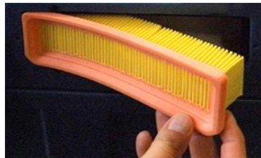
Fig. 8: Air filter change
