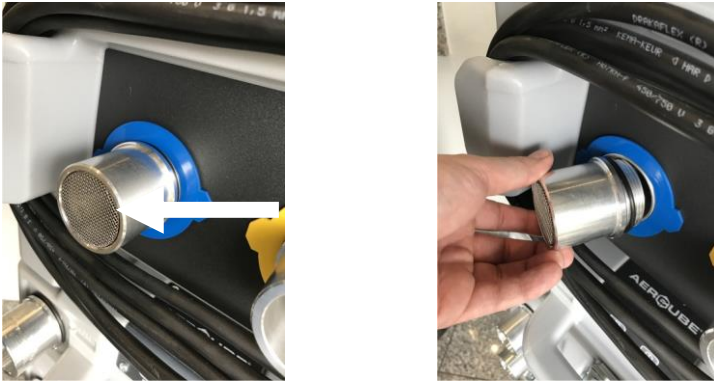
Fig. 9: Coarse filter intake socket
